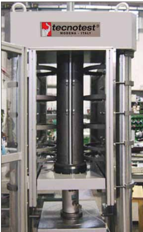
Calibration of the machine, using a load cell
