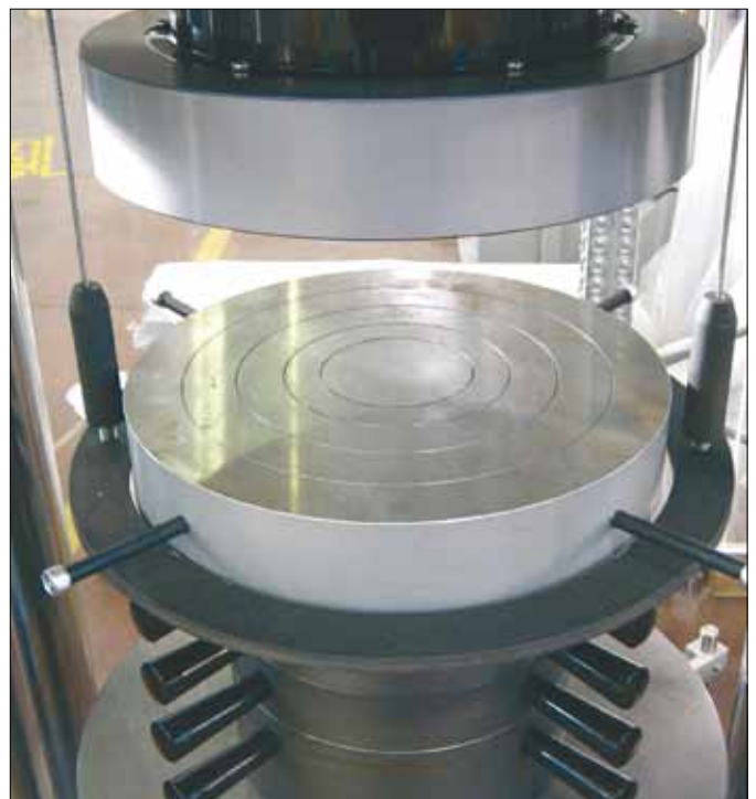
Mechanical lifting system of the lower platen ( KC 300/N - KC 300/ISP)
