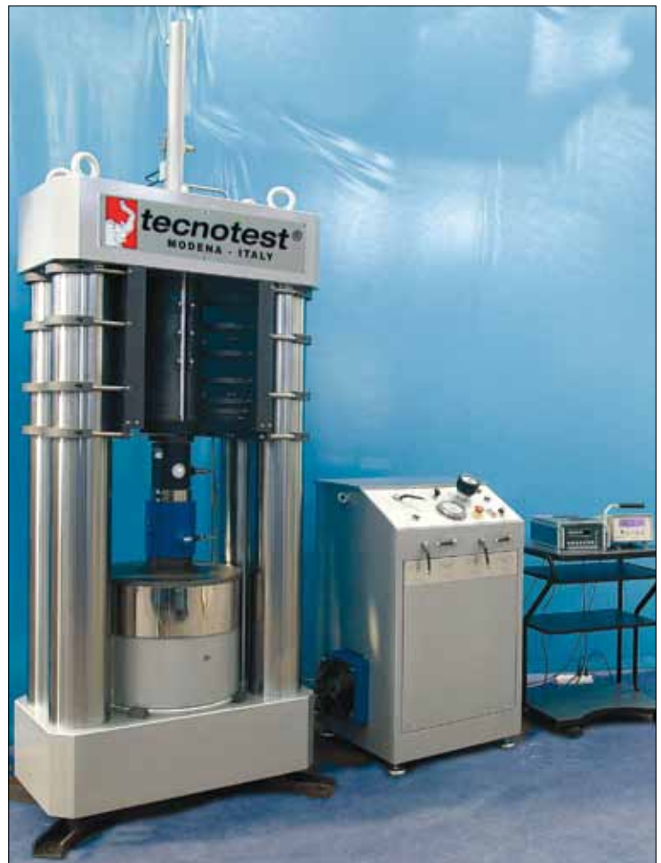
5000/600 KN MACHINE FOR CALIBRATING LOAD CELLS (COMPRESSION)
