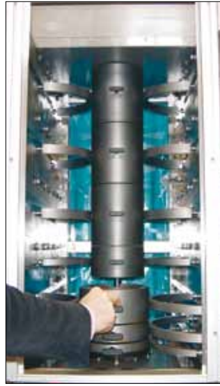
KC 300/S: Drawer system with 7 distance pieces for variation of the vertical testing span from 160 mm (min.) to 1000 mm (max.)
