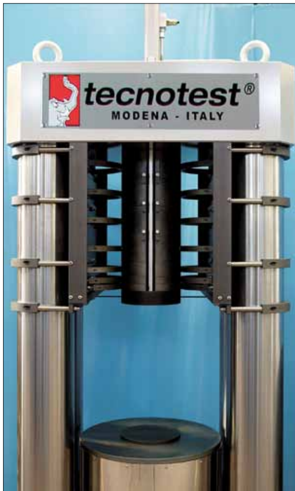
5000/600 KN MACHINE FOR CALIBRATING LOAD CELLS (COMPRESSION)
