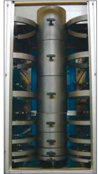
KC 300/S: Drawer system with 7 distance pieces for variation of the vertical testing span from 160 mm (min.) to 1000 mm (max.)
