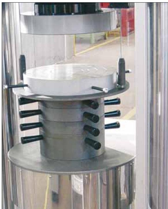
Mechanical lifting system of the lower platen ( KC 300/N - KC 300/ISP)
