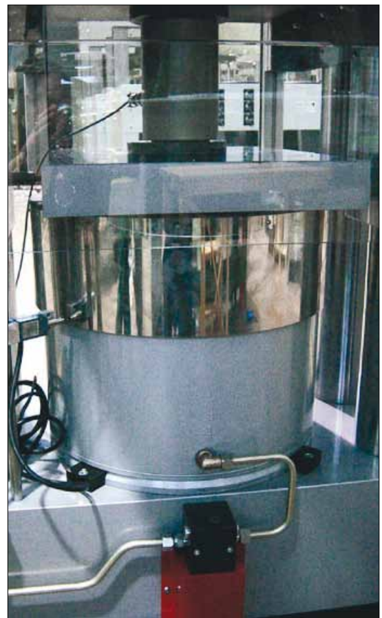
Hydraulic cylinder (295 bar max. pressure)
