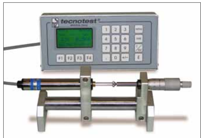
AD 161 WITH TRANSDUCER AND READOUT UNIT DURING CALIBRATION
