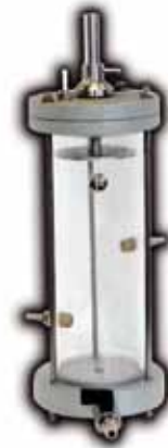
T 689 PERMEABILITY CELL diameter 75 mm Weight: approx. 3 kg
