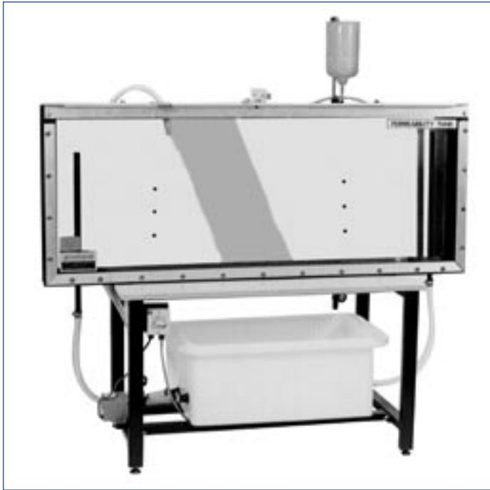
*Practical demonstration and visualisation are essential elements of fluid flow study. This Drainage and Seepage Tank has been designed to allow students to make an experimental study of flow through permeable media.*
